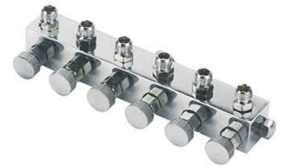
A9-6 6 Way manifold one G1/4 Female-Six 1/8 male Air flow adjustable
