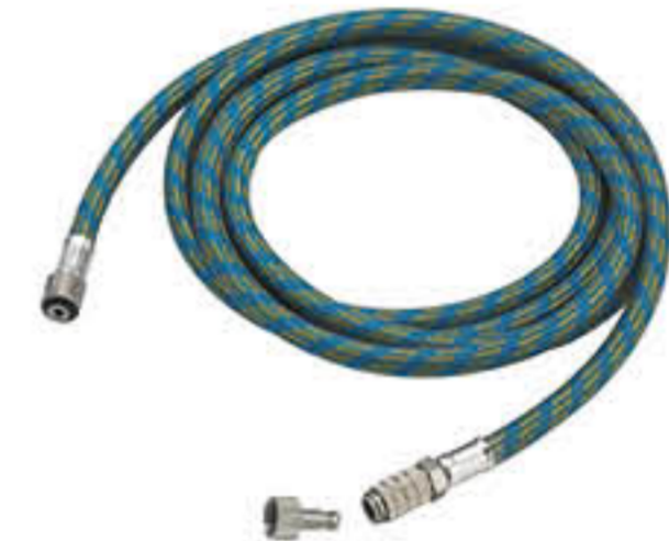
AH-27 Dia:7.5X4.5mm Length:1.8m(6ft),3m(10ft) Adaptor:G1/8"-G1/8" With the quick-release coupler
