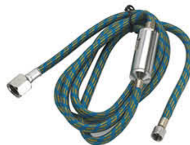
AH-26A Dia:7.5X4.5mm Length:1.8m(6ft),3m(10ft) Adaptor:G1/4"-G1/8" With the Filter
