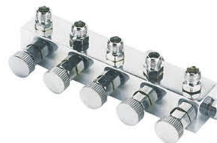
A9-5 5 Way manifold one G1/4 Female-Five 1/8 male Air flow adjustable
