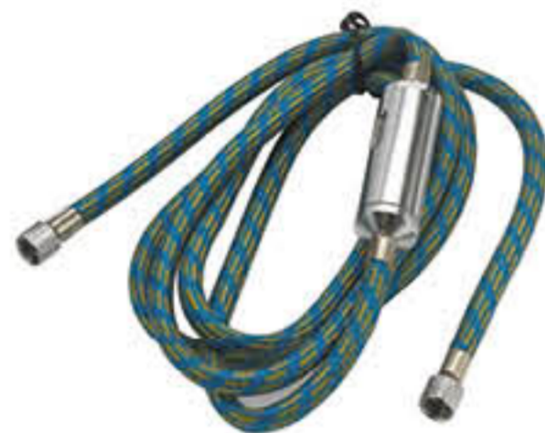
AH-26 Dia:7.5X4.5mm Length:1.8m(6ft),3m(10ft) Adaptor:G1/8"-G1/8" With the Filter
